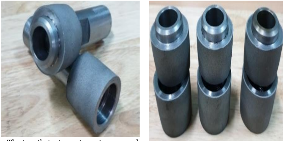
b. The tensile test specimen is removed from the shaft
