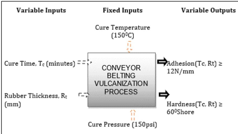
Figure 1. Illustrating the conveyor belting vulcanization process problem
