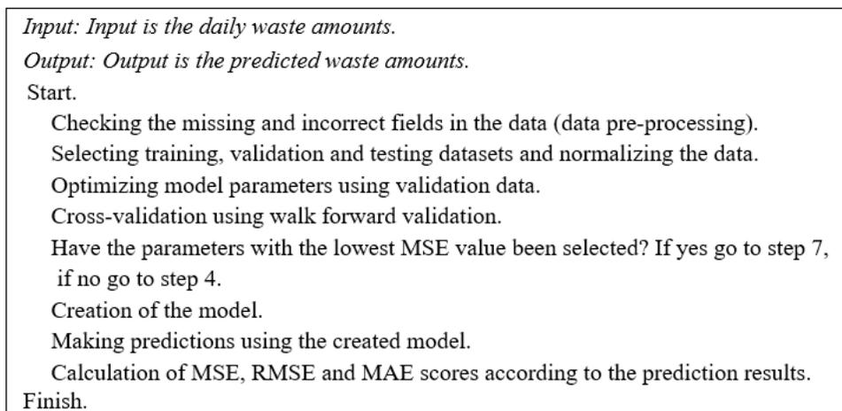
Figure 3. The algorithm of the developed system
