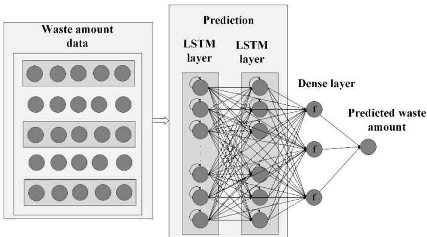
Figure 4. Developed LSTM-based deep learning model
